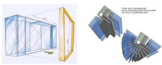
**project:** the actual owner desired a "light" addition facing the backyard: allowing maximum daylight to enter the living room, whilst respecting the building restrictions applied to the monument. the small extension is to be build, removed and rebuild within a single day: a galvanised steel structure is "clamped" between the brickwalls by means of a timber frame.
